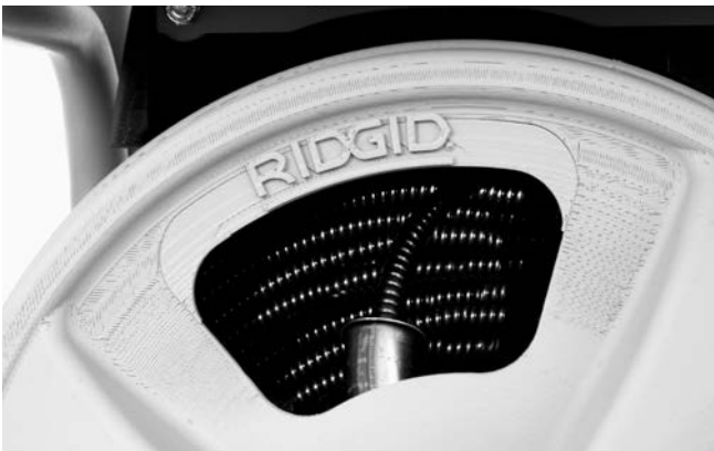
Figure 17 – Coil Cable Into Drum As Shown
