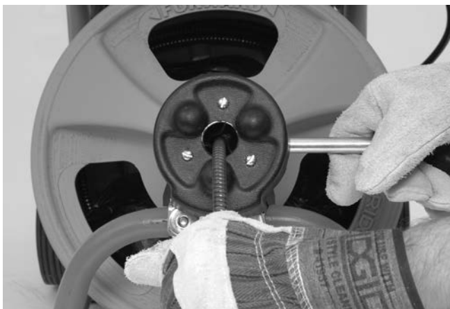
Figure 14 – AUTOFEED in Retrieve Position
