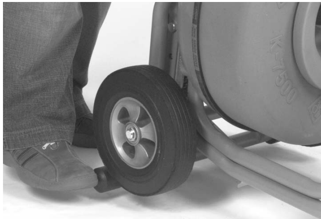
Figure 9 – Releasing Kickstand Bar
