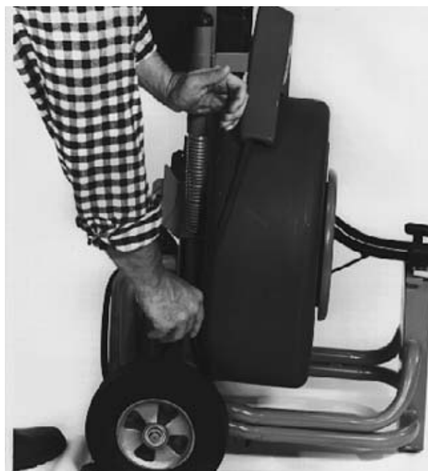
Figure 18 – Release Belt Tension
