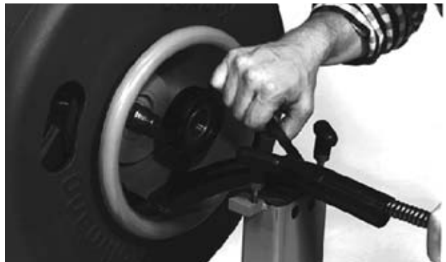
Figure 22 – Removing Guide Tube Assembly
