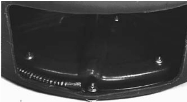
Figure 24 – Anchoring of Pigtail in Drum
