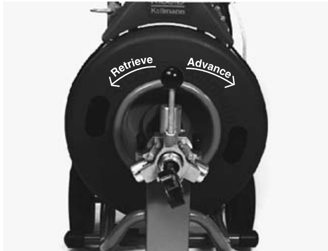
Figure 11 – Feed Lever Operation
