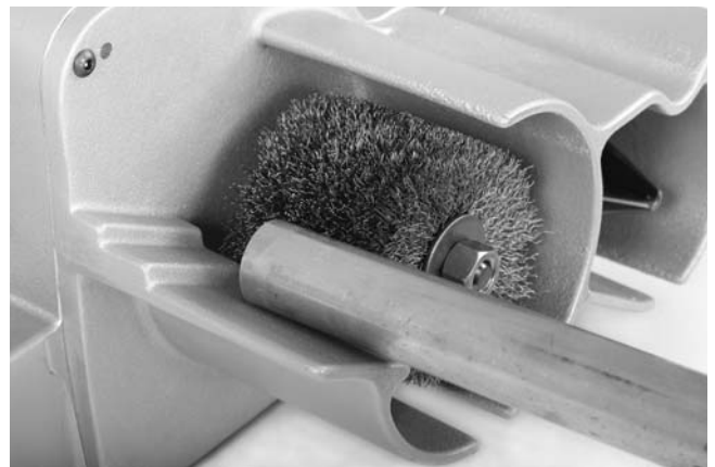
Figure 11 – Cleaning Tube O.D.
