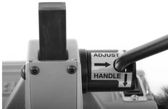
Figure 8 – Adjusting Handle Position
