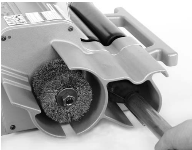
Figure 13 – Reaming I.D. of Tube
