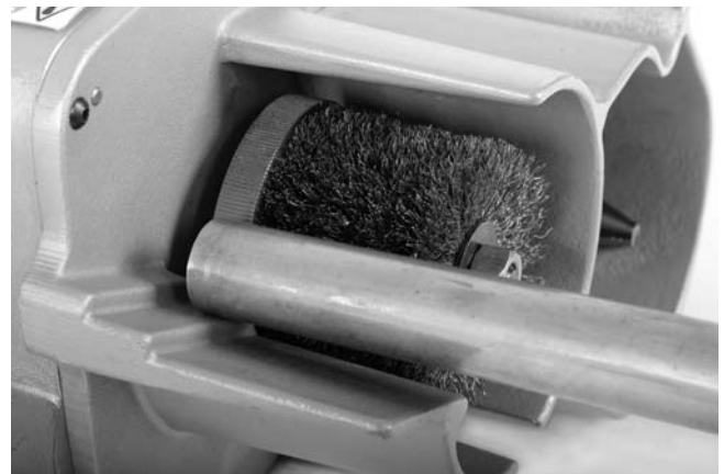
Figure 12 – Deburring O.D. Of Tube
