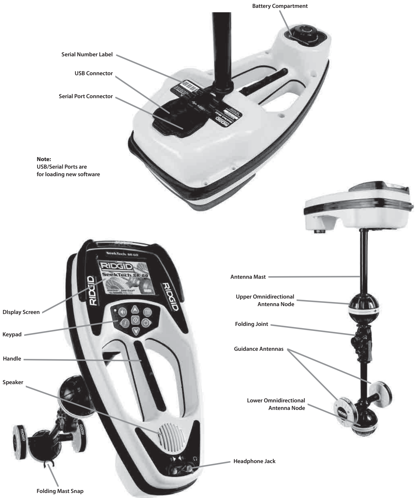
Figure 1: SR-60 Components
