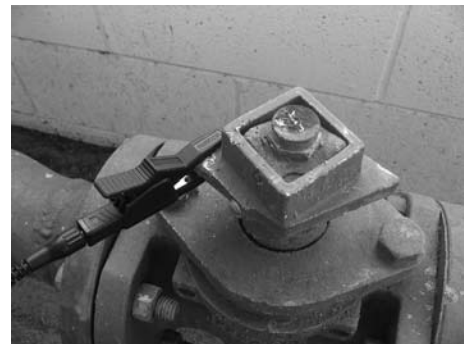
Figure 7: Connecting the ST-305 to a Line
