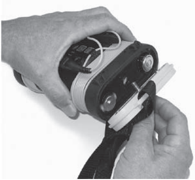
Figure 3: Removing the Battery Cover
