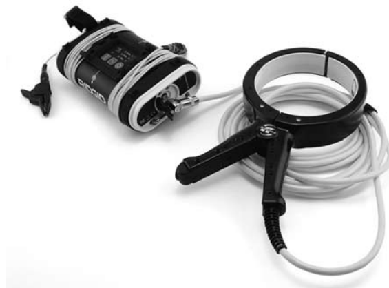
Figure 8: ST-305 with Inductive Clamp
