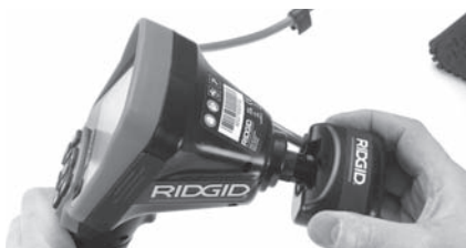
Figur 19 – Kameraets tilkopplingsplugg installert
